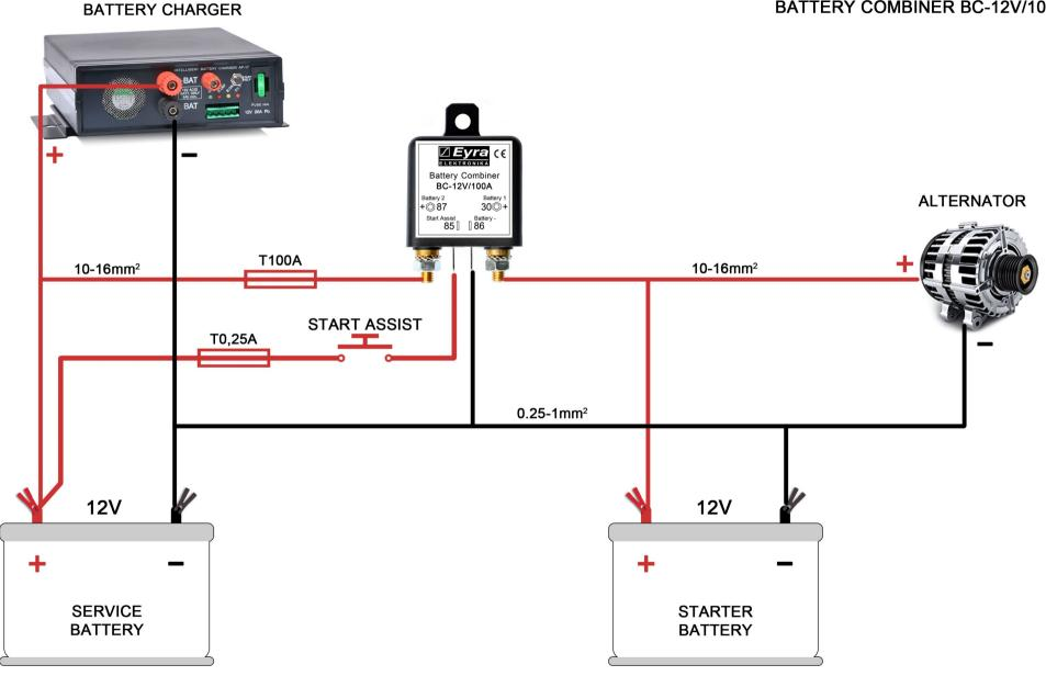
note: wire 10mm² for length\* 3m wire 16mm² for length\* 20m
