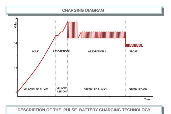
Pulse charging system is electrode specific charging system; it is new technology of battery charging. It presents a small revolution on this area, because the results in practice are drastically better. With this technology is possible very fast and very precise charging, because only electrochemical condition of battery "dictates" the
